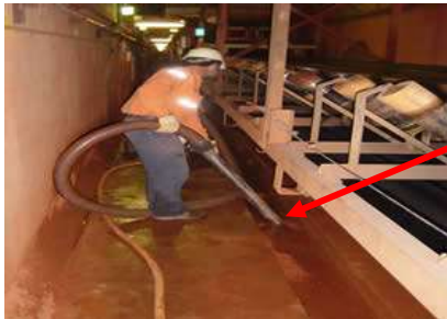
Showing valuable spilled product recovered and returned to belt.
