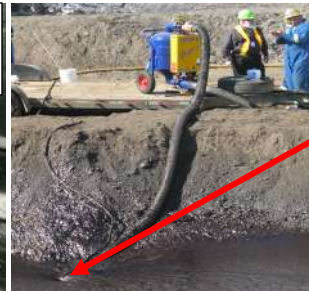
Showing valuable spilled product recovered and returned to belt.
