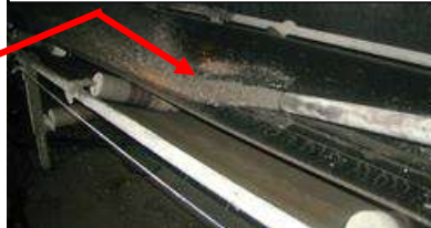
Spilled product is recovered and returned back to belt.
