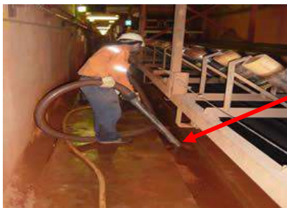
Spilled product is recovered and returned back to belt.
