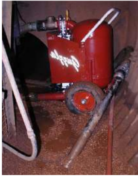
Typical mill water sludge lagoon with accumulated solids prior to mobilization of Supavac pump system. Vacuum recover settled sludge with hard solids with auto pressure discharge ~one kilometer as required.
