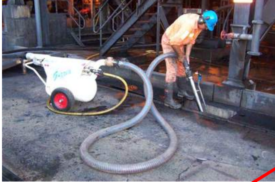
Typical mill water sludge lagoon with accumulated solids prior to mobilization of Supavac pump system. Vacuum recover settled sludge with hard solids with auto pressure discharge ~one kilometer as required.
