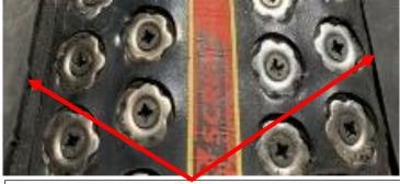
And now with a smooth and even top cover, no more damage to belt and screw fasteners, and scrapers can clean more effectively.
