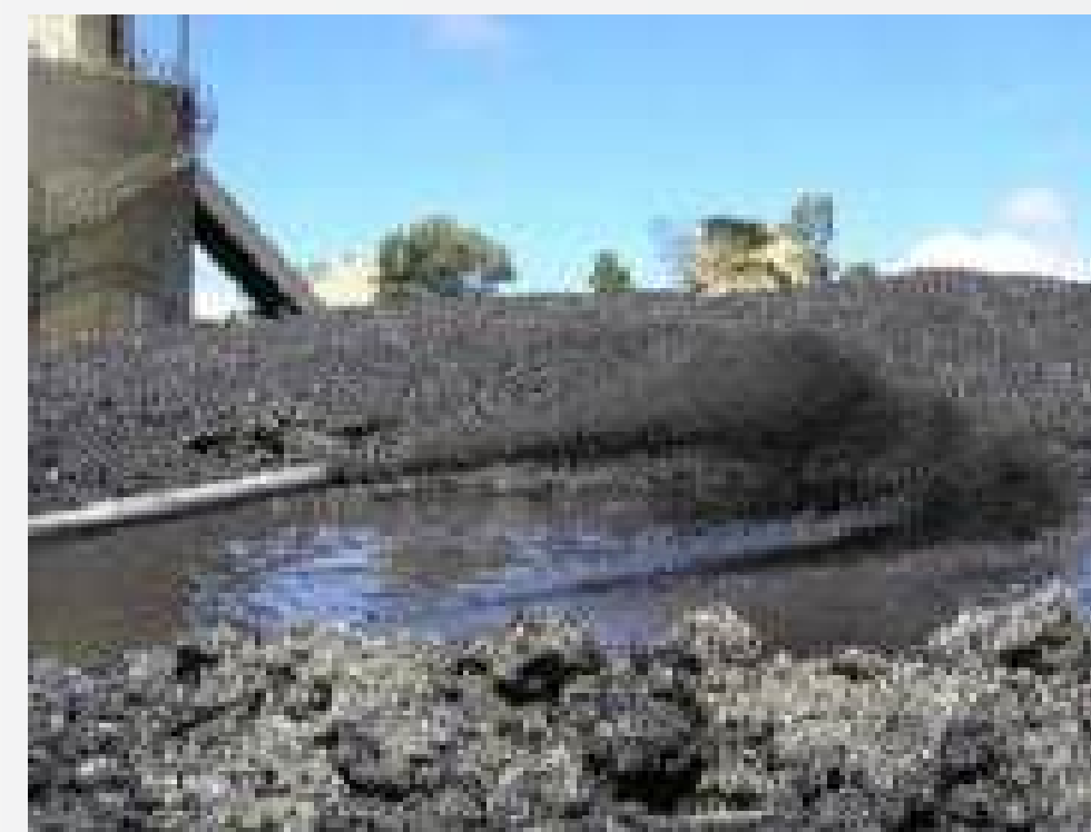
Solids can be discharged up to one km (1000s of ft) plus.
