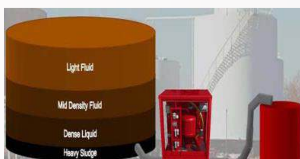
Accumulated settled hydrocarbon waste was removed from storage tank for disposal with zero leaks.
